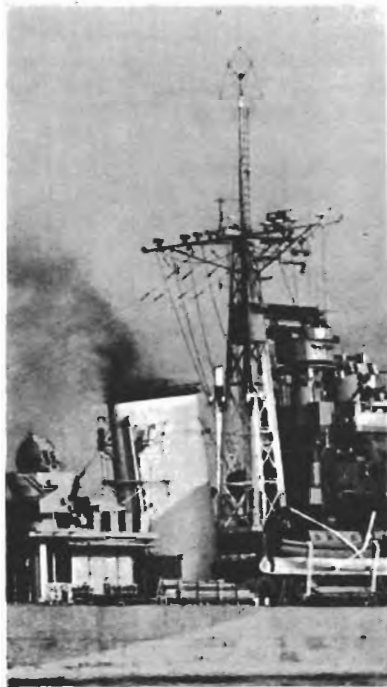
Aerial for H/F Direction Finder (Fixed Crossed Loop) mounted at top of Foremast on Destroyer
